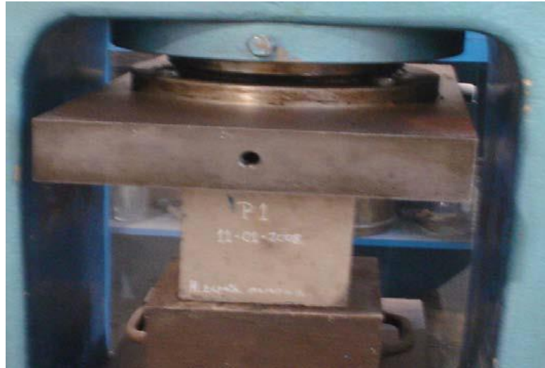
Figure 2.6. Barraza [24] performed a simple compression test on a cubic mortar sample
