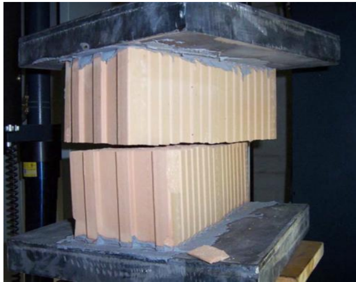
Figure 2.10. Tensile bond test for brick-mortar transition point [18]
