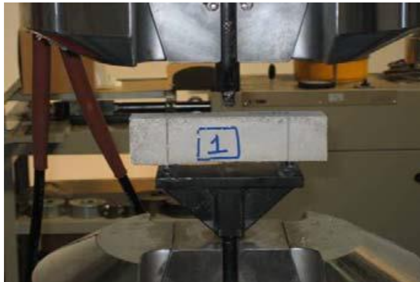
Figure 2.7. A mortar specimen is subjected to a flexural tensile strength test [21]
