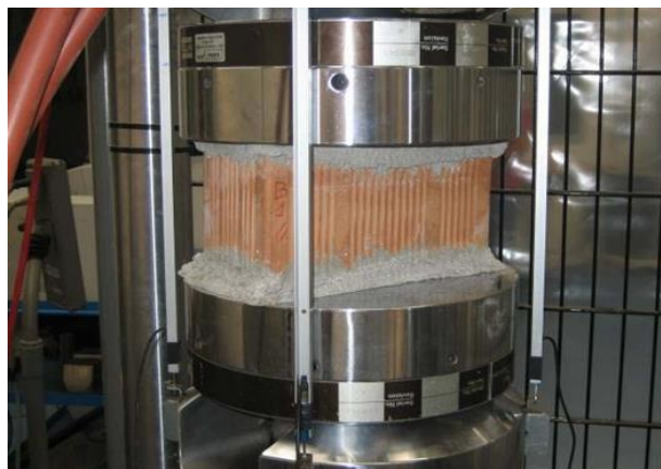
Figure 2.1. A brick specimen is subjected to a simple compression test [21]
