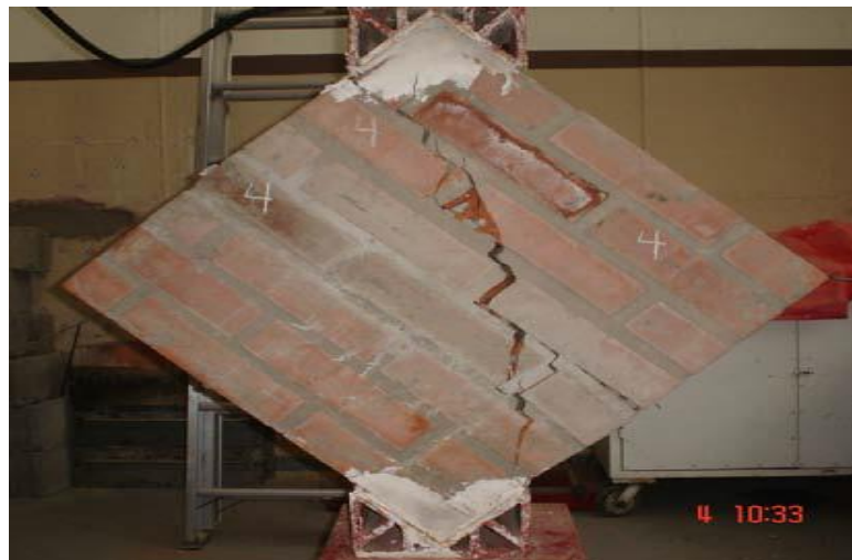
Figure 2.13. Diagonal compression test for a wall sample [24]
