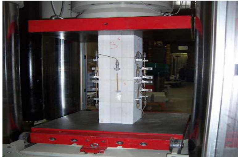
Figure 2.12. A Rilem brickwork specimen is put through a compression test [18]
