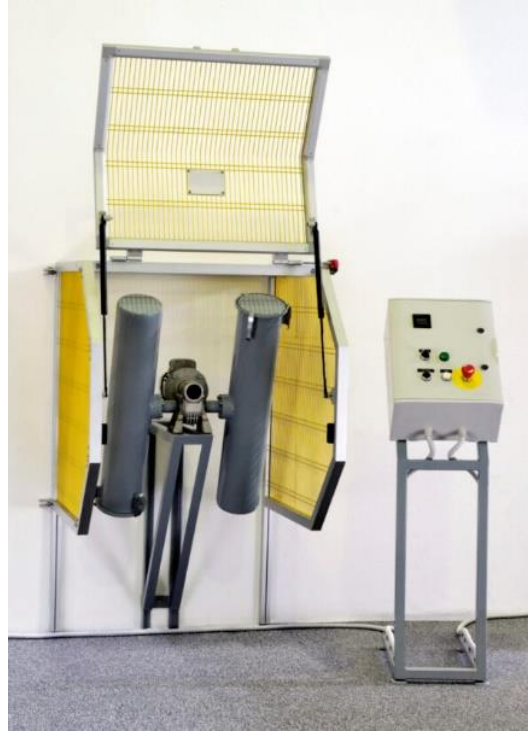
Şekil 4.9. CSR (Coke Strength after Reaction) tamburu [30]
