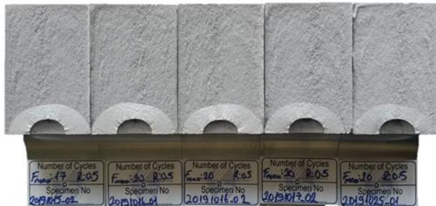
Figure 4.34. Fracture surfaces from 3-D fatigue crack growth tests under R=0.5 constant amplitude
