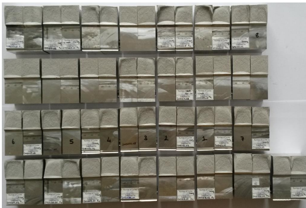
Figure 3.9. Top view of the used specimens for fracture tests
