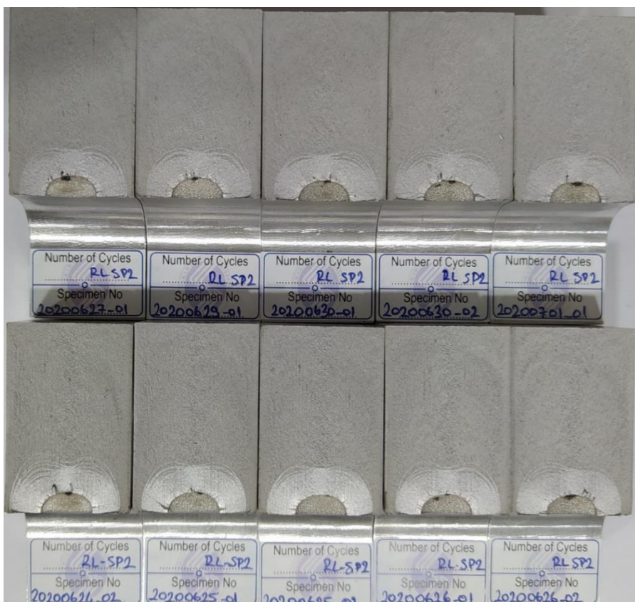
Figure 4.41. Fracture surfaces occurred under Spectrum-2 loading for 3-D FCG
