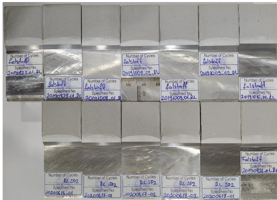
Figure 3.29. Fracture surfaces of the specimen tested under Spectrum-2
