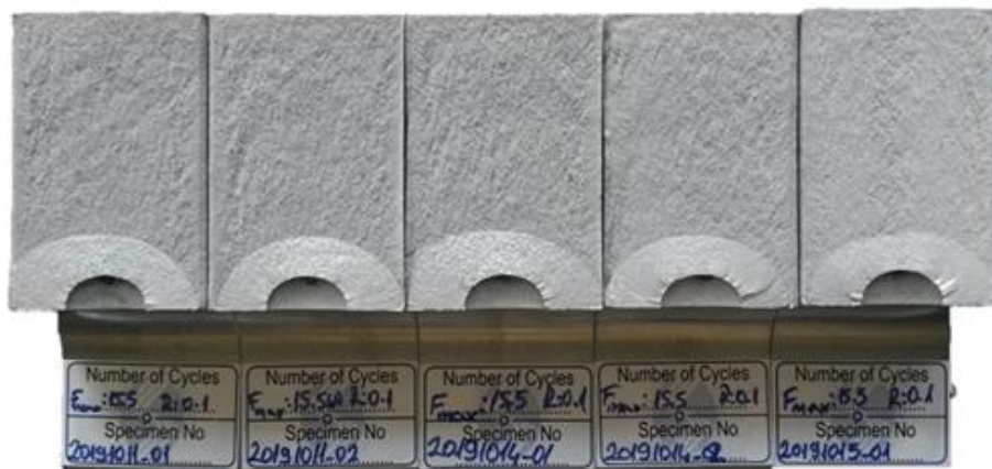
Figure 4.33. Fracture surfaces from 3-D fatigue crack growth tests under R=0.1 constant amplitude
