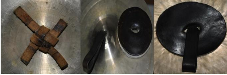
Figure 4. How to attach the cymbal handle
