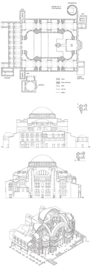
Figure 5: Plan, elevation, section and axonometric views of Hagia Sophia (12)
