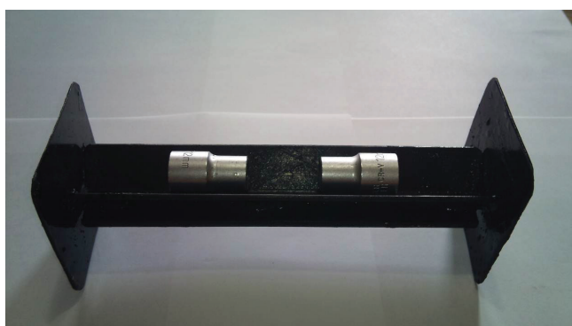
Figure 4. A sliding mold system that has been used to center the bones in the mold until satisfactory hardening of the cement is achieved
