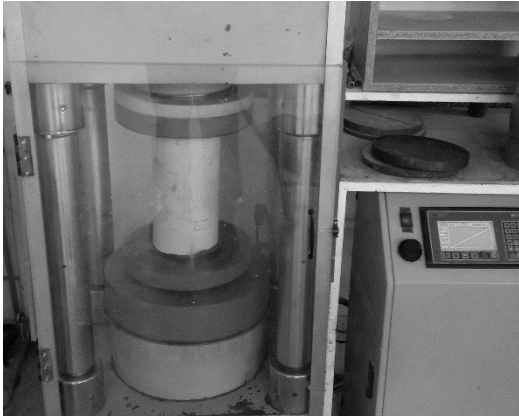
(a) Beton presi
