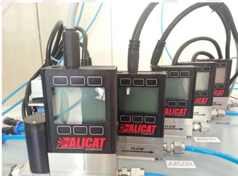
Figure 5.5. Mass flow meters used for regulating gas flow into the measurement cell
