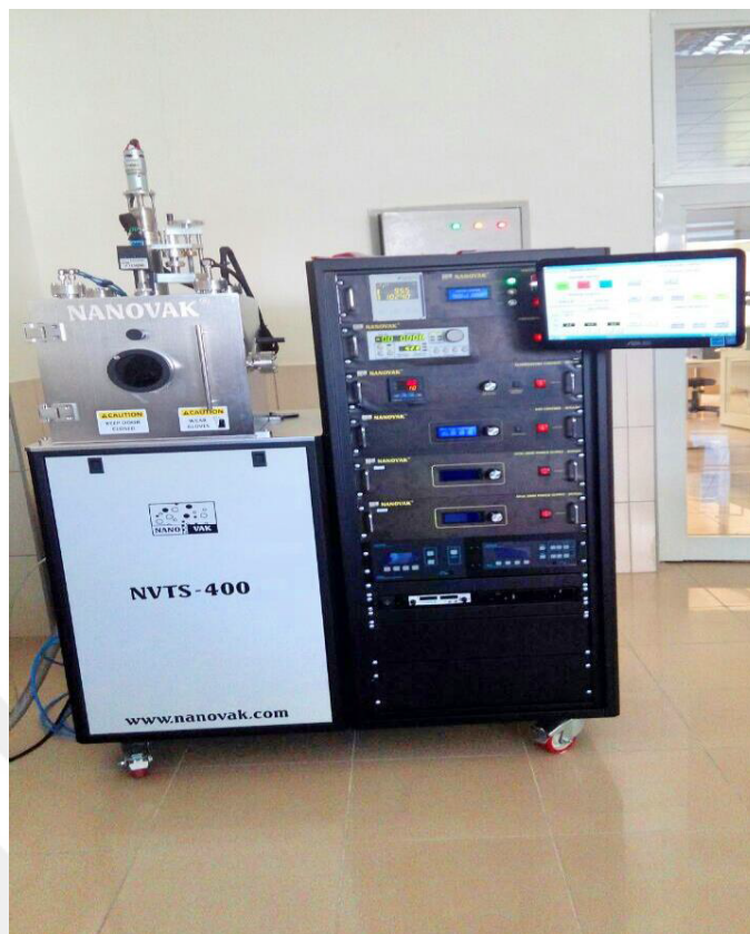
Figure 5.1. Magnetron sputter system at Nigde University
