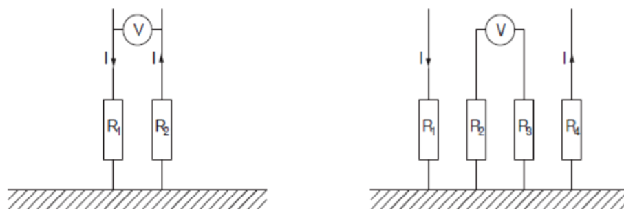
Figure 4.11. The set-up comparison of the two probe and four probe system [69]
