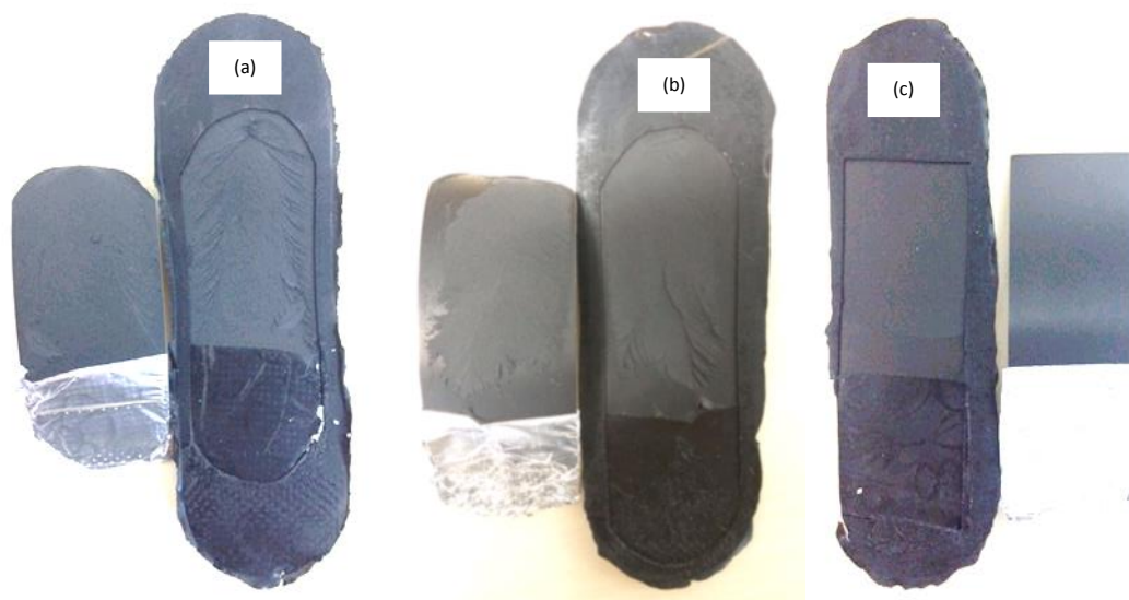
Figure 6.19. Images of the interface adhesion failures between Chemosil coated aluminum and EPDM surfaces after T-peel strength test. (a) Cohesion failure of EPDM at 100 °C for 2, 4, 8, 16 and 64 min. and 165 °C for 2 and 4 min., (b) Partially adhesion and cohesion failure at 165 °C for 8 min., (c) Adhesion failure at 165 °C for 16 and 64 min.
