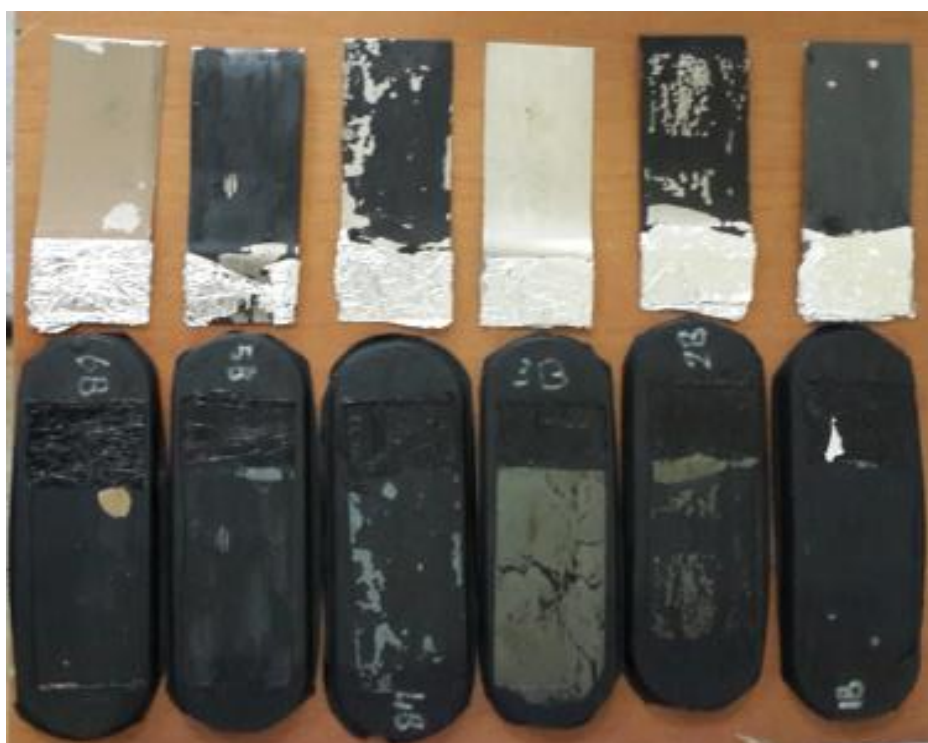
Figure 6.41. Images of the interfaces of “B” series coating applied between aluminum stripe and EPDM based rubber plate after T-peel test.
