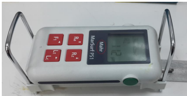
Figure 5.8. Mahr MarSurf PS1 surface roughness measurement device.
