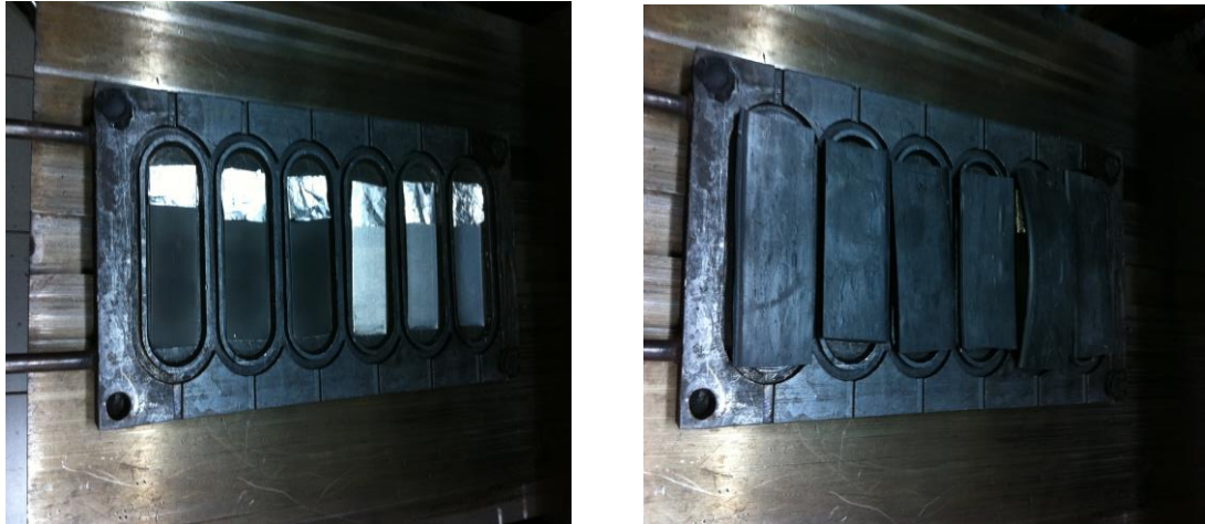
Figure 5.5. Sample holder used in the molding step.
