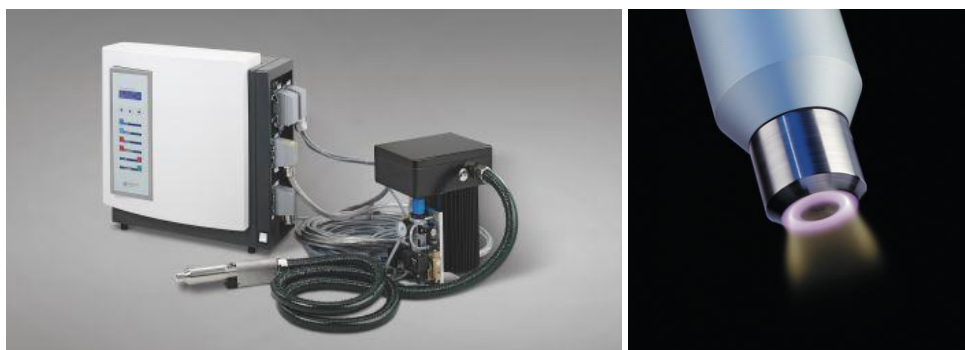
Figure 5.3. The plasma treatment unit and plasma nozzle [47].
