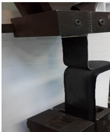
Figure 5.9. T-peel strength test of the interface of EPDM based rubber compound and Al strip.
