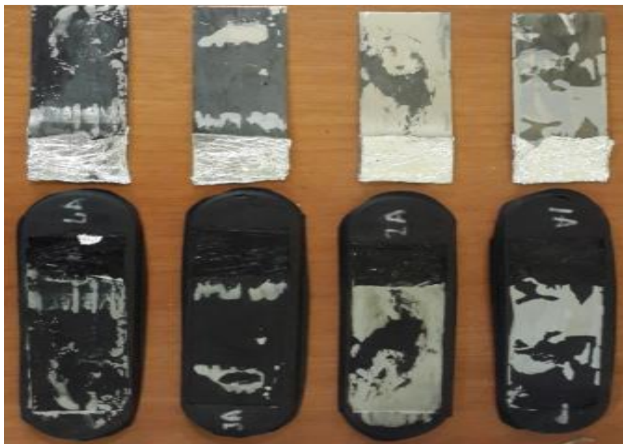
Figure 6.40. Images of the interfaces of “A” series coating applied between aluminum stripe and EPDM based rubber plate after T-peel test.
