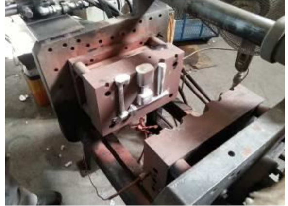
Fig. 1. A mold after the die casting process.
