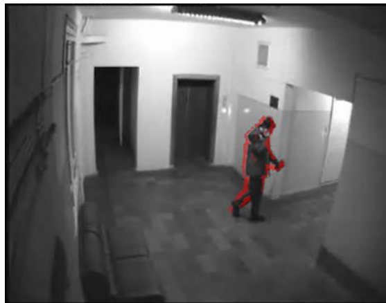
Figure 2.1. Two frames difference motion detection [20].
