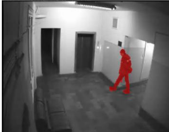
Figure 2.2. Simple background modeling motion detection [20].
