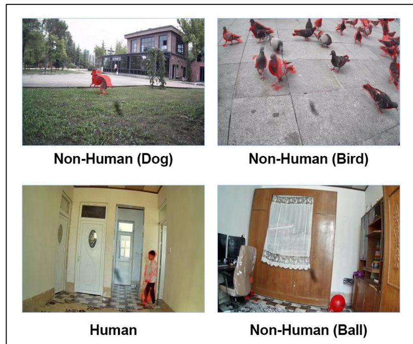
Figure 4.7. An example of motions determined by the system using TFDA and Tiny YOLOv2.
