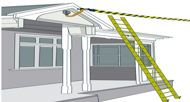
Figure 5.4. Overhead LV Connections.
