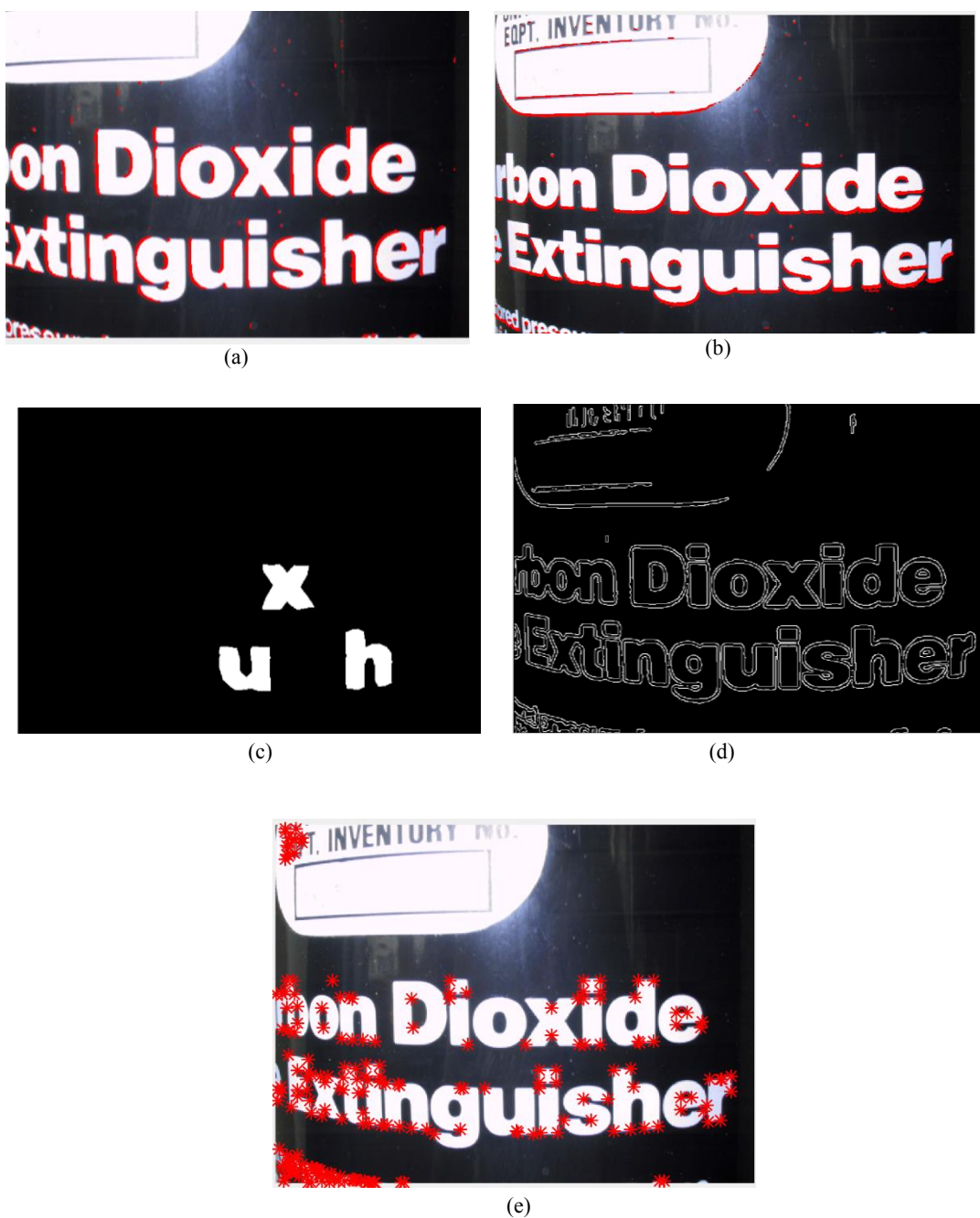
Figure 4.1. High and low transitions (a) and (b), interest regions (c), edges and boundaries (d) and corners (e).
