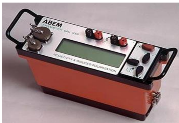
Figure 4.1. Image of ABEM Terrameter SAS 1000C (Anon 2011)
