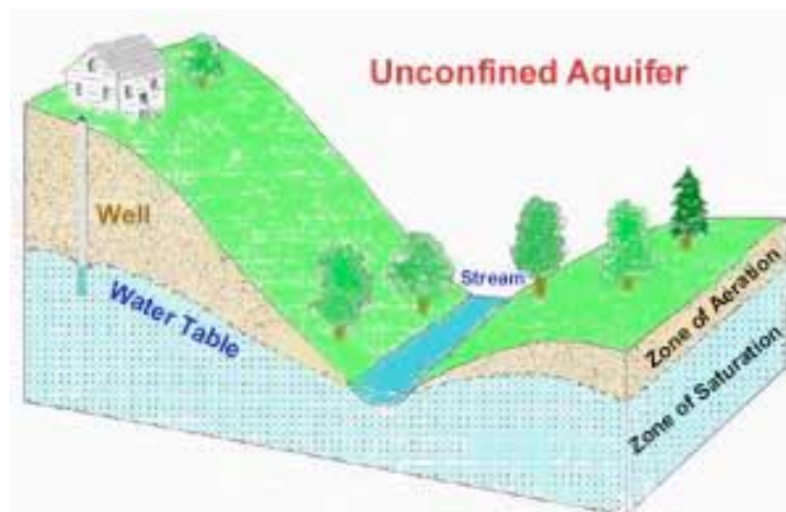
Figure 2.4. Schematic cross-section of unconfined aquifer ( obtained from Groundwater Storage (Anon n.d.))
