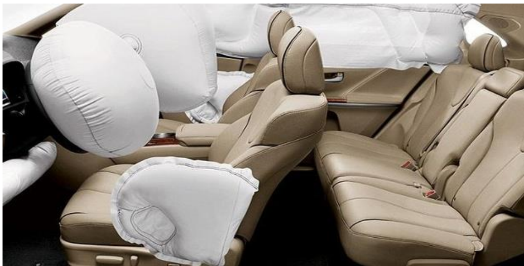
Figure 1.15. Air bag system in the car
