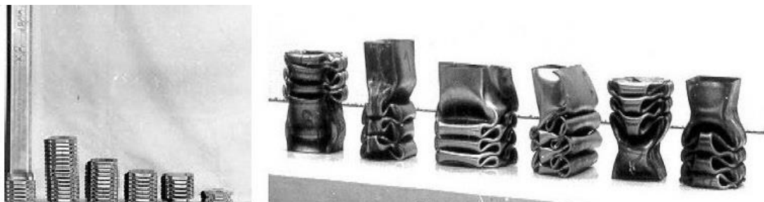
Figure 1.5. Folding of properly triggered elements, often subjected to axial impact loading
