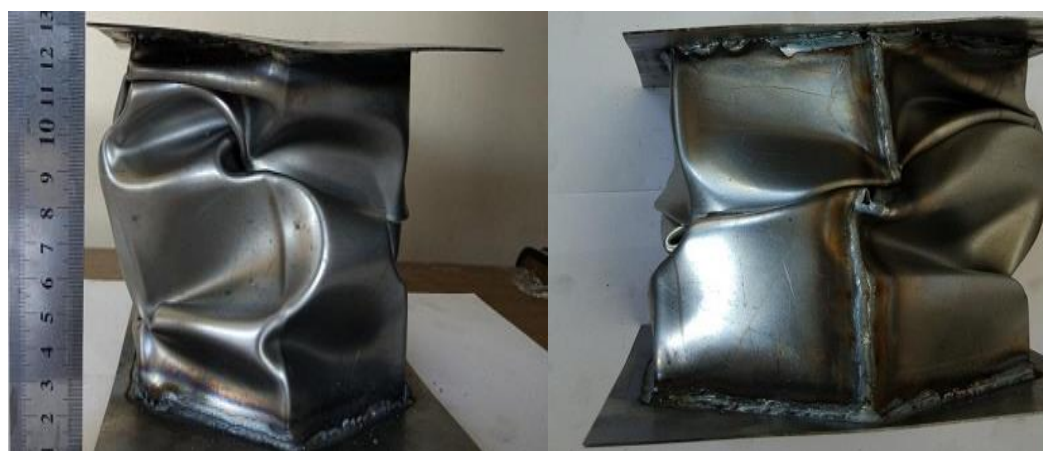
Figure 4.29. 250mm height of sample after deformation and weld zone of Hexagonal Profile
