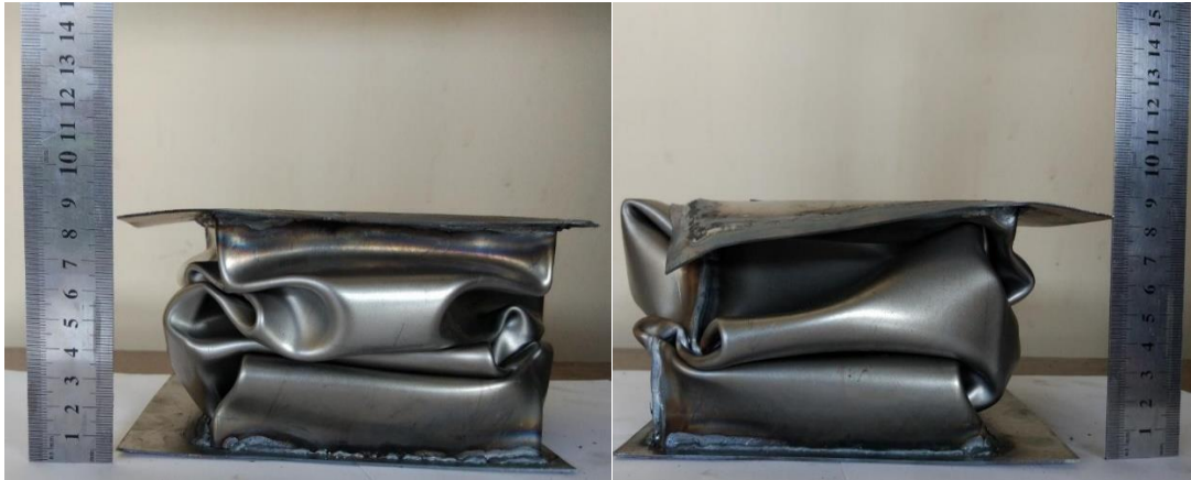
Figure 4.32. 250mm height of the sample after deformation and weld zone of Square Profile
