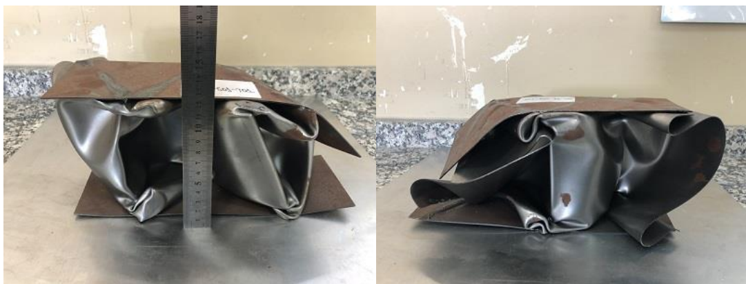
Figure 4.16. W02-II.0-S01-T01 sample's front and back view after collision
