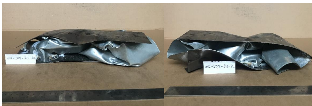
Figure 4.19. W02-I0.8-S01-T01 sample's front and back view after collision
