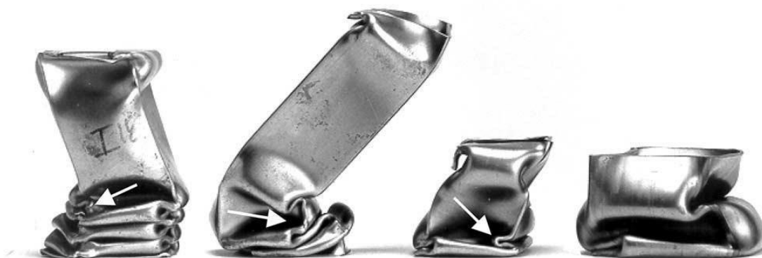
Figure 1.6. Square columns resulting from the development of symmetric and 'inverted' folding modes indicated by white arrows
