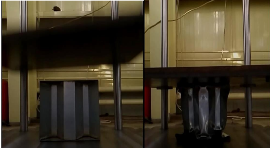
Figure 4.4. W01-I1.5-S01-T01 sample slow motion recording photographs when the drop plate hit the crash-box
