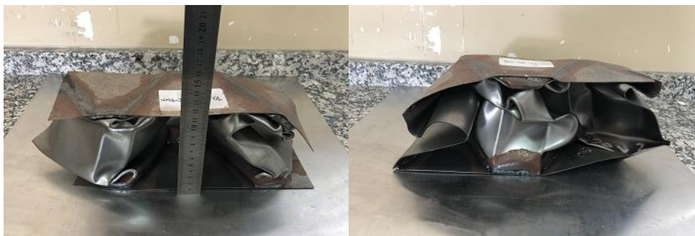
Figure 4.8. W01-II.0-S02-T01 sample after deformation Front & Back side view
