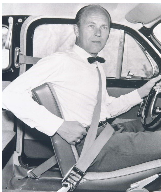
Figure 1.14. Safety engineer Nils Bohlin shows the 3-point seat belt used in 1959 Volvo cars
