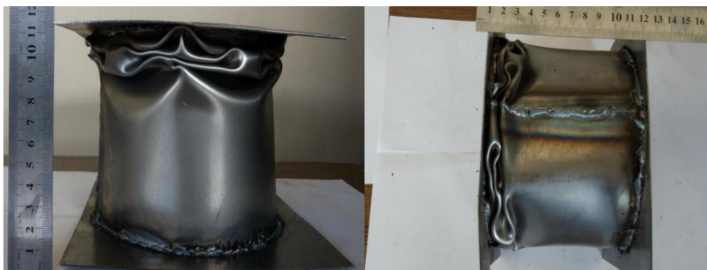
Figure 4.27. 200mm height of the sample after deformation and weld zone of Circle Profile
