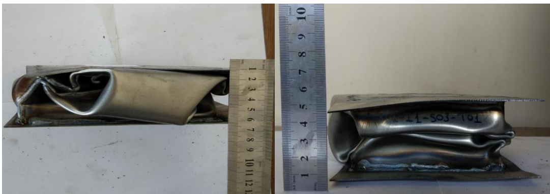
Figure 4.33. 200mm height of the sample after deformation and weld zone Square Profile
