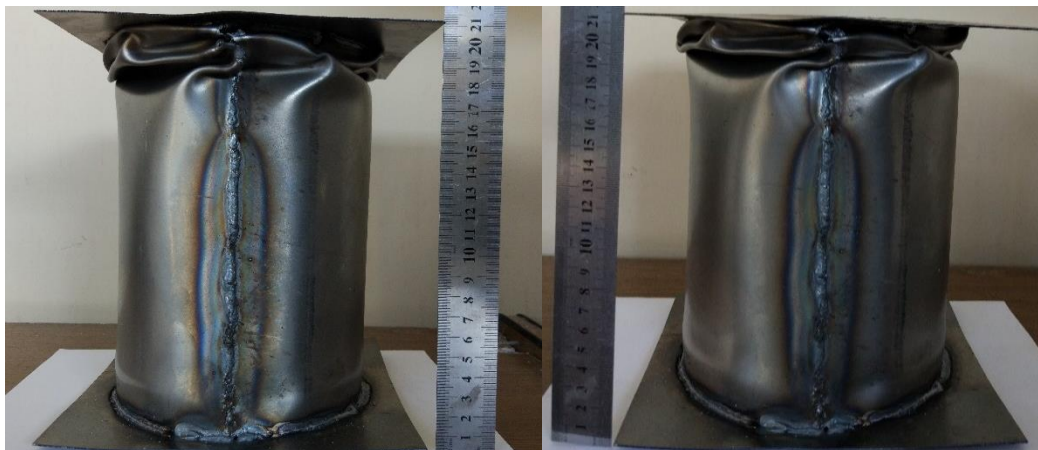
Figure 4.25. 300mm height of the sample after deformation and weld zone of Circle Profile
