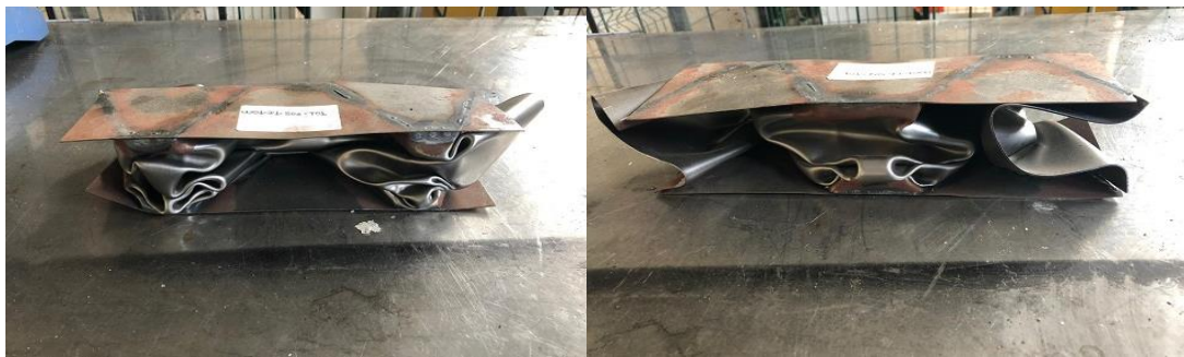
Figure 4.9. W01-II.0-S03-T01 sample after deformation Front & Back side view
