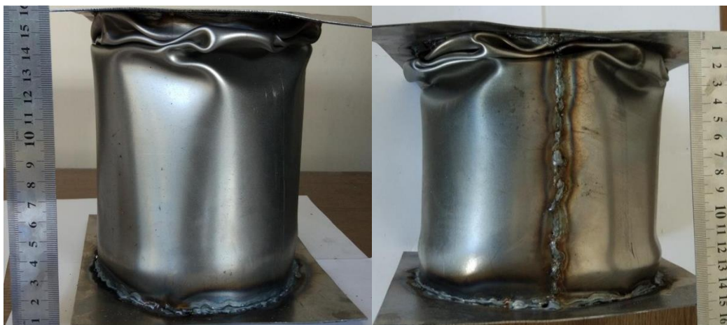
Figure 4.26. 250mm height of the sample after deformation and weld zone of Circle Profile
