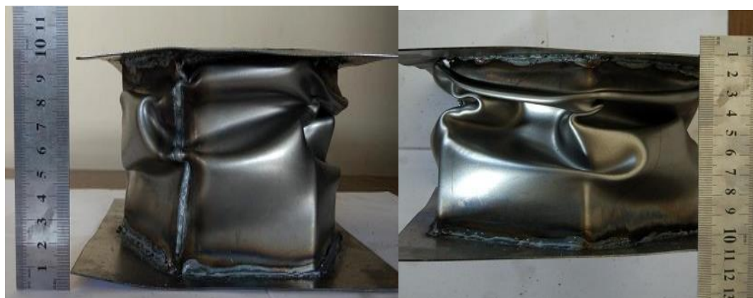
Figure 4.30. 200mm height of sample after deformation and weld zone of Hexagonal profile
