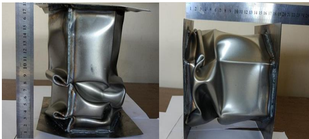
Figure 4.28. 300mm height of sample after deformation and weld zone of Hexagonal Profile
