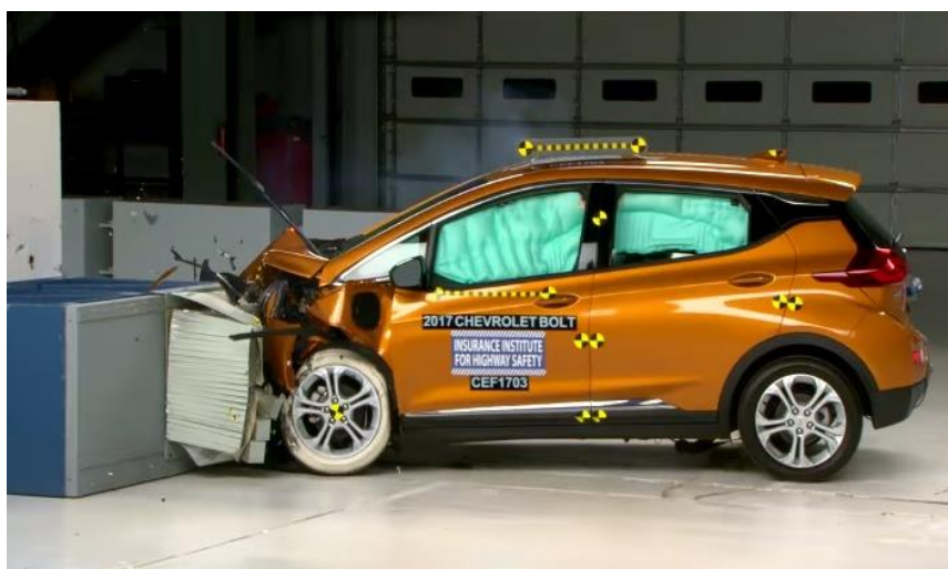
Figure 1.13. Crash Test of Chevrolet Bolt EV 2017
