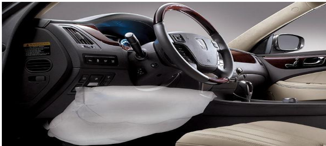
Figure 1.17. Knee airbag system in car
