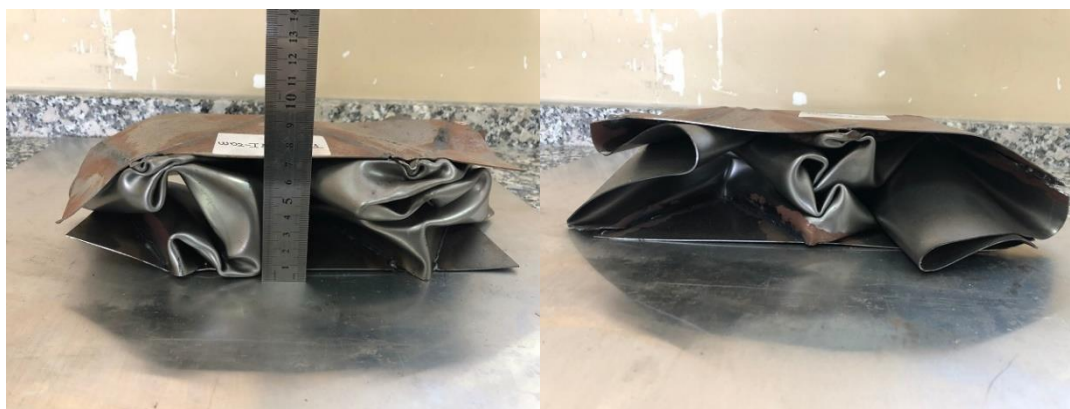
Figure 4.17. W02-II.0-S02-T01 sample's front and back view after collision
