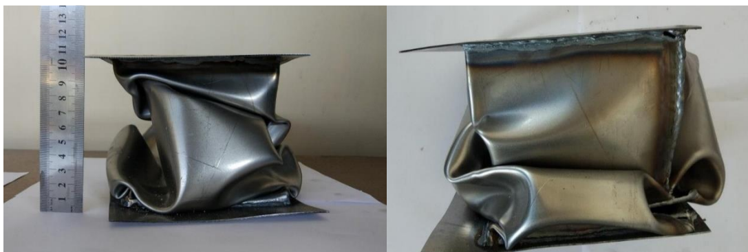
Figure 4.31. 300mm height of the sample after deformation and weld zone of Square Profile
