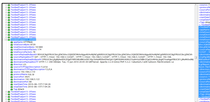
Figure 4.2. XML representation for a random anomalous network trace with its relevant profile captured during the 15th of June auditing activity.
