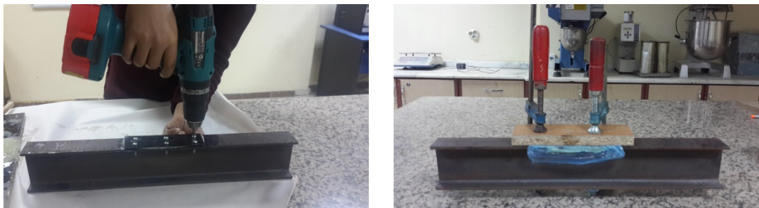
Figure 3.20. Employing bolts & clamping the specimens.
