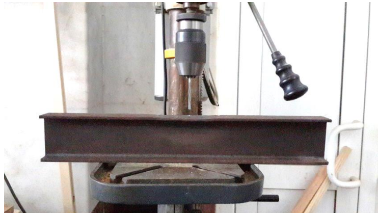
Figure 3.18. Drilling procedure for steel beam.
