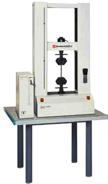
Figure 3.23. AG-IC Table-Top type UTM [53].
