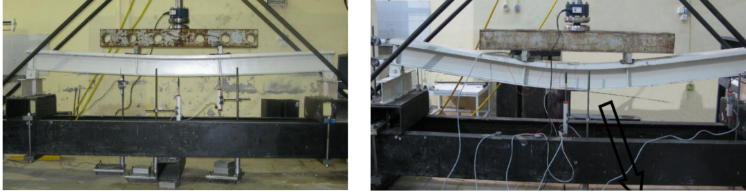
Figure 2.7. HM-CFRP strengthened composite I girder [32].
