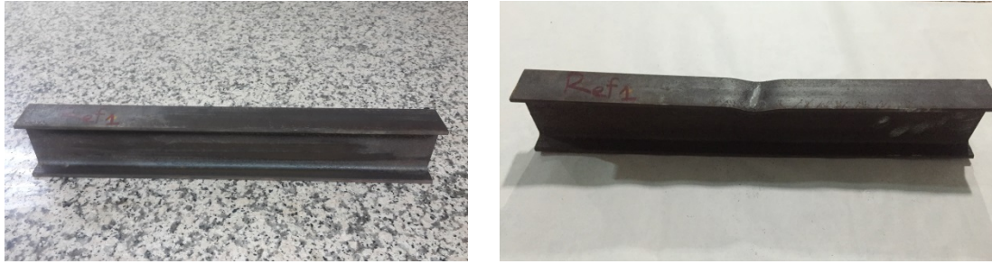
Figure 4.7. Reference beam before and after the test.
