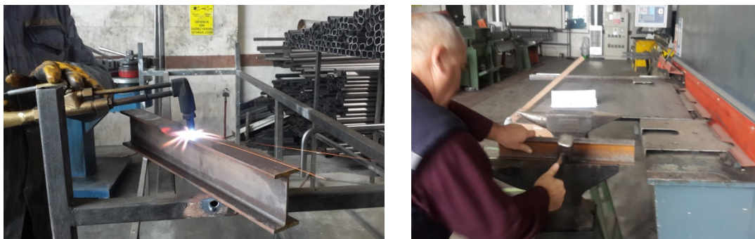
Figure 3.16. Heat treating and straightening of specimens.
