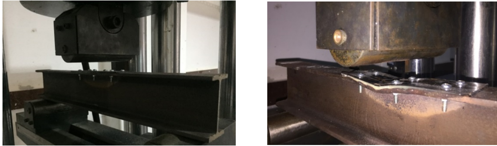
Figure 4.9. Retrofitted beams under three-point bending test.
