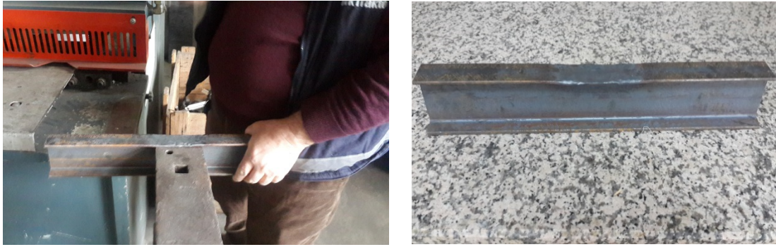
Figure 3.17. Straightened and heat-treated shape of test specimens.
