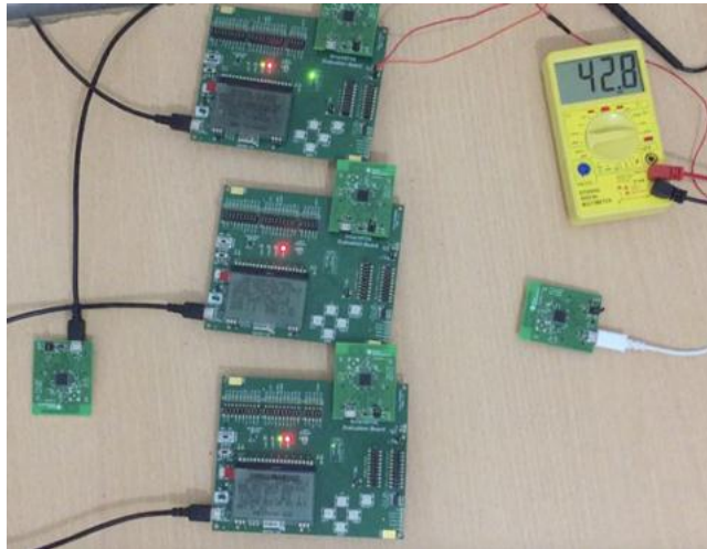
Figure 5.13. Measuring drawn current
