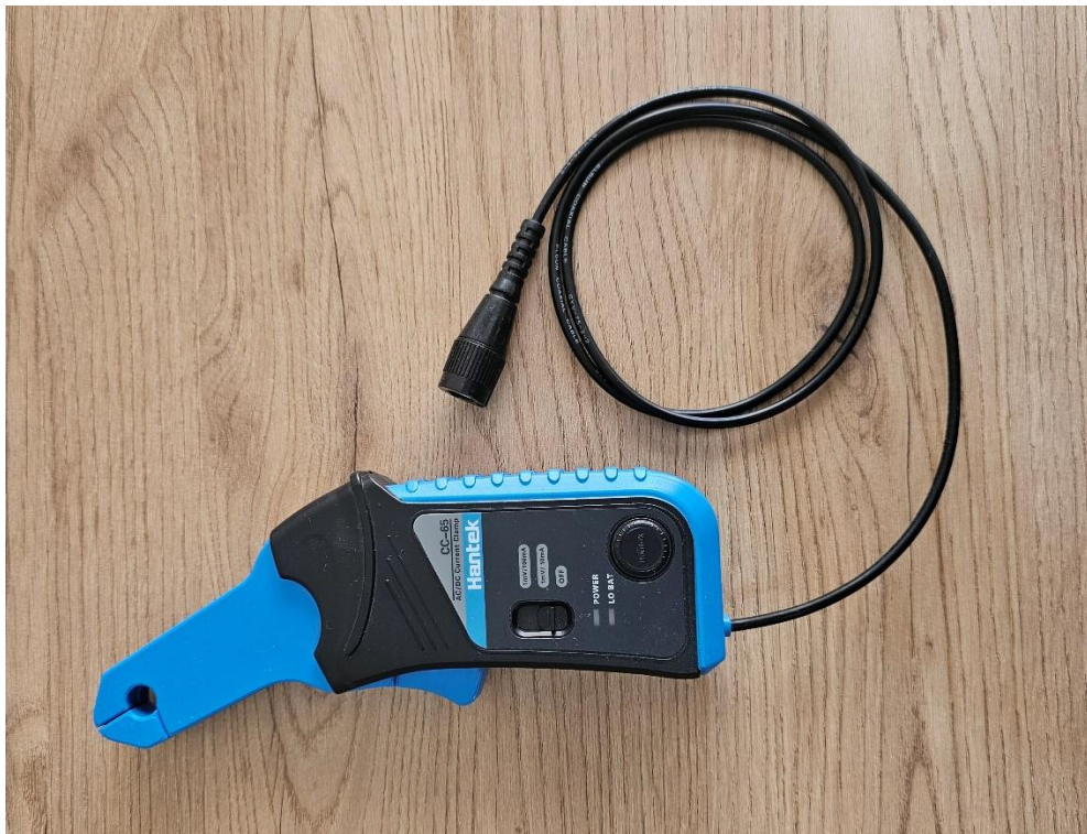
Figure 4.10. The practically used current measurement probe.
