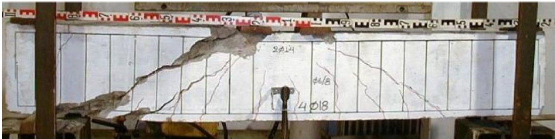
Figure 4.6. Damaged condition of ST80 beam after the test
