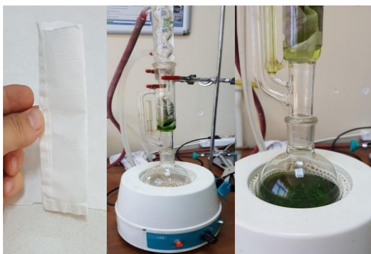
Figure 3.4. Preparation extract of Equisetum arvense L. By soxhlet method.
