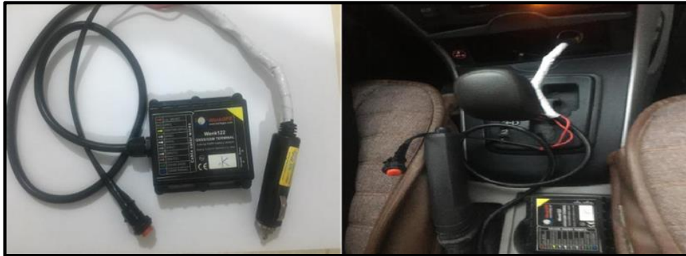
Figure 3.3. The manufactured GPS device.
