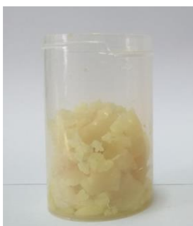
Figure 4.6. The obtained solid PBZ polymer after decontamination step
