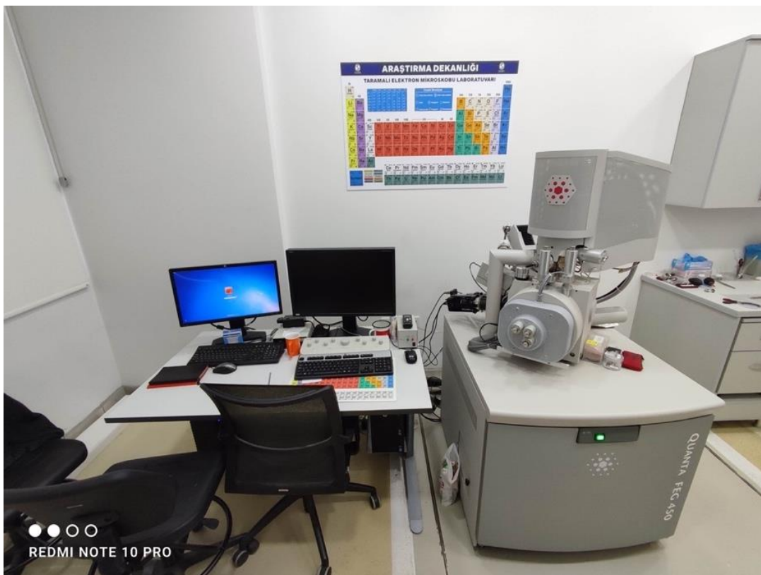
Figure 3.14. FESEM used in the characterization of the synthesized powders.
