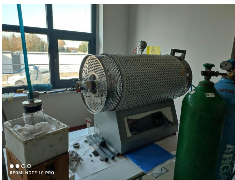
Figure 3.9. The DTM modified rotary furnace.
