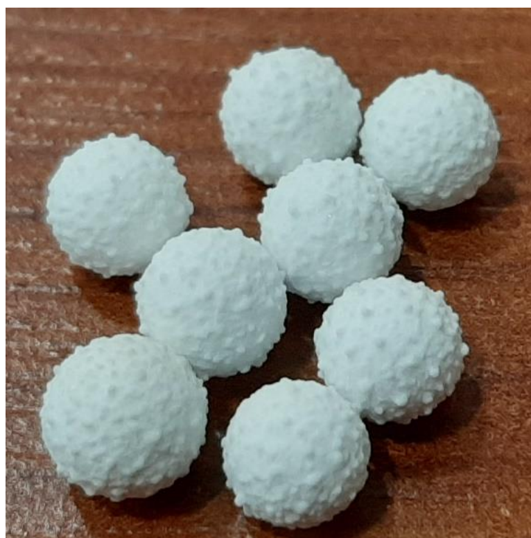
Figure 4.8. Alumina balls after being used in the synthesis of spinel powder at 1500°C for 1.5h with at 2rpm. (B/P was 20.) Satellite formation clearly visible on the balls indicates alumina deposition.
